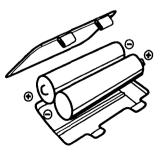
**NOTE:** If the unit suddenly stops working or the sound becomes weak turn the unit off for 15 seconds, then turn it back on. If the problem persists it may be caused by weak batteries. Please install a new set of batteries and try the unit again.
